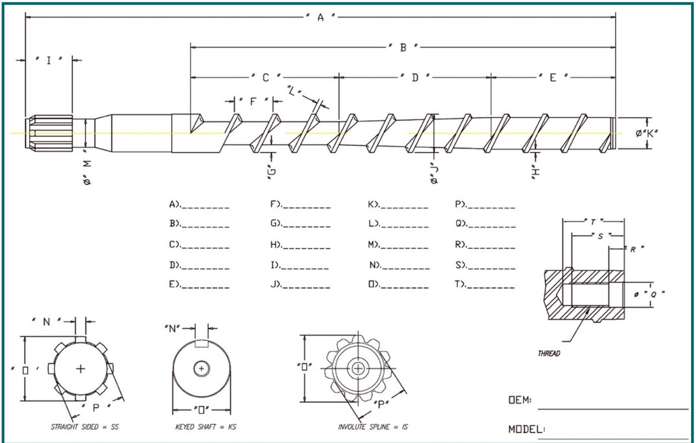
**The screw configuration plays a critical role in the plasticization process (drawing courtesy of Cooper Technology)**
